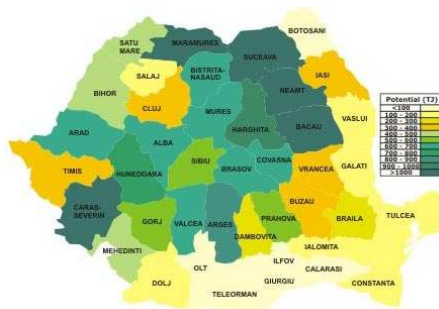
Figure 3 - Energetic potential allocation of biomass in Romania.
